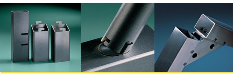
Adding "tabs and slots" in varying forms to mating components can drastically reduce the amount of secondary operations required to form strong, accurate joints between parts.
