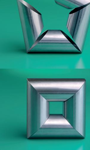
Designing for the laser process allows a radius corner to be created from a square or rectangular tube forming an aesthetically pleasing and "safe corner" on furniture etc.
